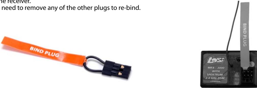
3. With the Bind plug installed, turn on the vehicle. You will notice a blinking LED within the receiver.
