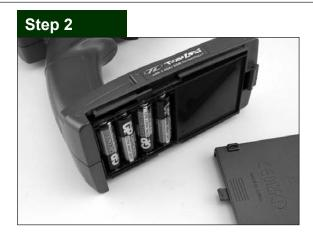
Remove the transmitter battery cover by sliding the cover from left to right. Install four (4) AA batteries into the battery holder. Pay close attention to the correct direction of the positive (+) and negative (-) ends as marked in the tray. Once all 4 batteries have been installed, reinstall the battery cover by sliding it on from right to left.
