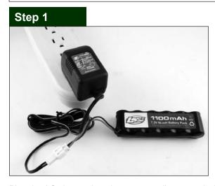
Plug the AC charger into the proper wall receptacle (110V). Plug the battery pack into the charger and let it charge for 3 hours for the first time. After running, or when the Mini-Slider slows noticeably, recharge the battery pack for 5 to 6 hours for a full charge.
