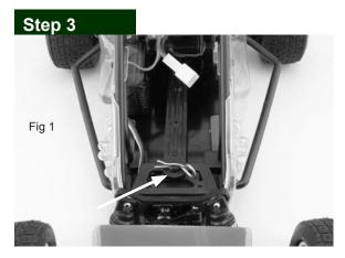
Once the battery is charged, remove the body clip from the front battery hold down and remove the battery strap (fig. 1).
