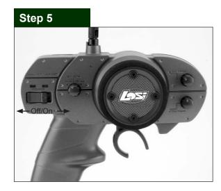
Always turn on the transmitter first by sliding the switch on the left side of the wheel from left to right. The small red and green lights above the switch should both light up. If not ,you need to check for low or incorrectly installed batteries.
