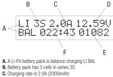
**F.** Time elapsed since the charge process started is 22:43 (22 minutes and 43 seconds) During charging, the Dec key can be pressed to show several parameter messages on the LCD screen including: End Voltage, Capacity Cut-off, Safety Timer setting, Temperature Cut-off and
