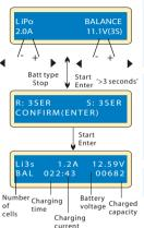
The left side of the first line shows the type of battery you have selected. The value on the left side of the second line is the current you have selected. After setting the current and voltage, press the 'START/ENTER' key for more than three seconds to start the process (charge current: 0.1-5.0A, voltage: 3.7-22.2V)
