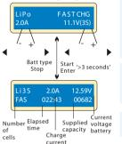
As the charger reaches the end of the charging cycle, the charging current will drop. A specific CV process will be reduced to end the charging process earlier. In fact, the charging current will drop to 1/5 when the charging process comes to 1/10. Charging capacity will be less than normal charging, but charging time will be shortened accordingly.
