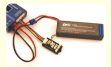
The main battery leads must be connected along with the balance lead connectors as shown before charging your battery. Pay close attention to the polarity of the main battery leads.
