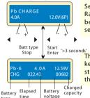
Set up the charge current on the left and nominal voltage on the right. Range of charge current is 0.1-5.0A, the voltage should match the battery being charged. Press and hold the 'START/ENTER' key for more than three seconds to begin charging.
