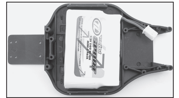
Battery Position “Forward”
