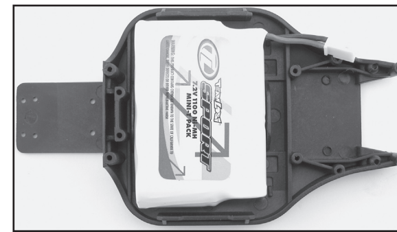
Battery Position “Back”
