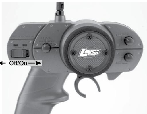
Always turn on the transmitter first by sliding the switch on the left side of the wheel from left to right. The small red and green lights above the switch should both light up. If not, you need to check for low or incorrectly installed batteries.
