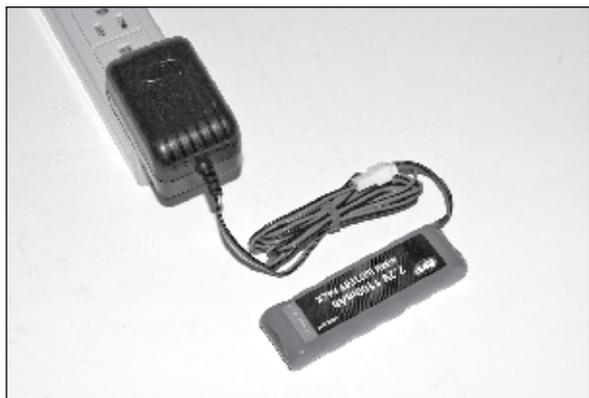
Choose the correct adaptor for your country and plug the charger into the proper wall receptacle. Plug the battery pack into the charger and let it charge for 3 hours for the first time. After running, or when the Mini Sprint slows noticeably, recharge the battery pack for 5 to 6 hours for a full charge.
