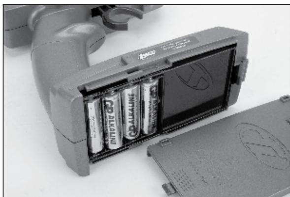
Remove the transmitter battery cover by sliding the cover from left to right. Install four (4) AA batteries into the battery holder. Pay close attention to the correct direction of the positive (+) and negative (-) ends as marked in the tray. Once all 4 batteries have been installed, reinstall the battery cover by sliding it on from right to left.
