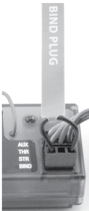
Although set at the factory, below are the steps required to re-bind your transmitter to the receiver should the need arise. During the bind process there is a unique ID from the transmitter communicated to the receiver to ensure trouble-free radio operation.
