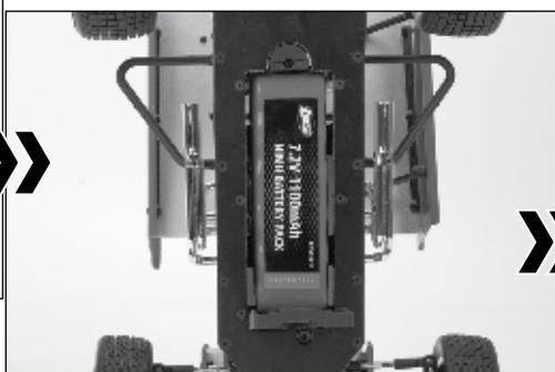
Insert the power leads through the opening in the back of the battery box as you install the battery. Close the door and turn the lock 1/2 turn to lock it shut.
