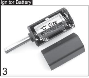
Remove the cover from the glow plug ignitor. Install a "C" size alkaline battery with the "+" end of the battery as shown in the figure above.
