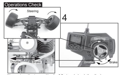
Always turn the transmitter "on" first and check the display screen for adequate voltage. Turn on the model and check both the throttle and steering for proper operation and battery power.
