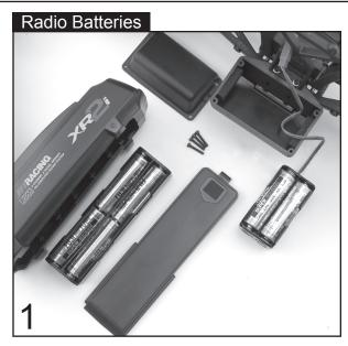
Refer to Figure 91 in the Owners Manual to install the radio antenna on the truck. Install the radio system batteries, 8 in the bottom of the transmitter and 4 into the back of the model as shown. Use only quality alkaline or rechargeable Ni-Cad AA-size cells.
