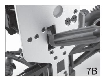
To stop the engine, use a rag to cover the exhaust pipe exit(fig. 7A) being EXTREMELY careful not to burn your hand as this will be hot, or use the handle of a screwdriver (fig. 7B) against the engine flywheel.
