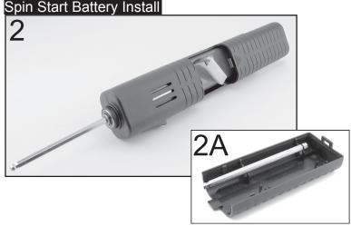
Slide back the battery access panel opposite the hand strap and remove the cover. Remove hex starter shaft from the back side of the cover (fig 2a.) and press the o-ringed end into the drive cup. Slide a 7.2 volt 6 cell "stick pack" into the Spin-Start and plug it in. Note that the plug is made such that it can be plugged in one way. Carefully tuck the plug wires under the battery access panel and slide shut.
