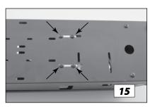
Disconnect the wires from the motor and mark the location of the mounting screws before removing. Remove the screws on either side of the wheel shaft. After replacing the wheel, be sure to re-install the assembly in its original position.
