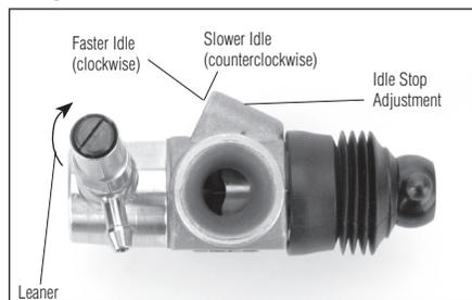
High-Speed Needle: 3 turns out (counterclockwise) from closed.
