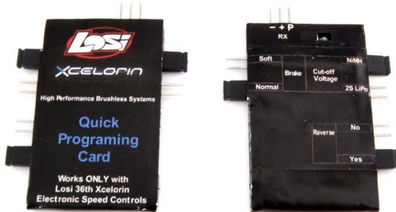
The supplied Quick Programming Card (QPC) is used to setup the Electronic Speed Control to your operating requirements.
