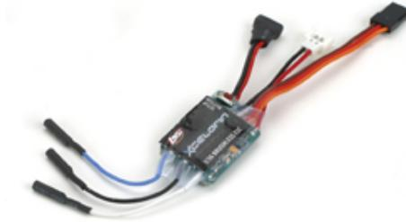
The ESC has connectors installed and ready for your use. The motor will connect to the ESC Motor wires by matching colors, Blue to Blue, White to White and Black to Black. Doing this the motor will run the proper direction for your Losi Micro Vehicle. Should you need the motor to operate in the opposite direction just disconnect any two of the connectors and reconnect in reverse fashion.
