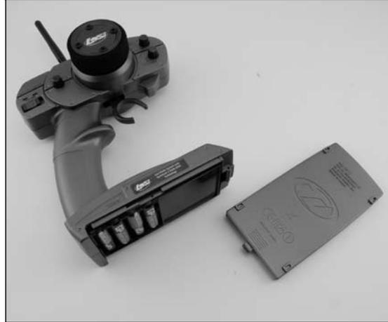
Remove the transmitter battery cover by sliding the cover from left to right. Install four (4) AA batteries into the battery holder. Pay close attention to the correct direction of the positive (+) and negative (-) ends as marked in the tray. Once all 4 batteries have been installed, reinstall the battery cover by sliding it on from right to left.
