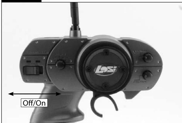
Always turn on the transmitter first by sliding the switch on the left side of the wheel from left to right. The small red and green lights above the switch should both light up. If not, you need to check for low or incorrectly installed batteries.
