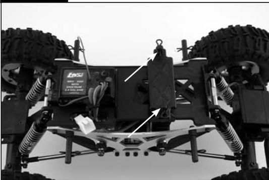
Once the battery is charged, remove the body clips from the battery hold-down and remove the battery strap (fig. 1).
