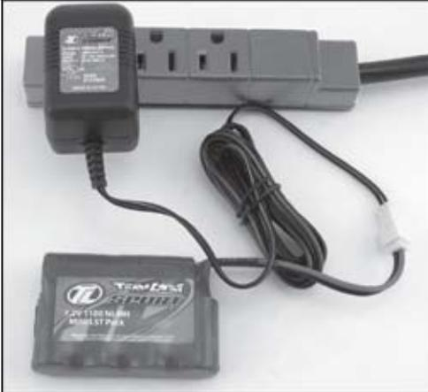
Plug the AC charger into the proper wall receptacle (110V). Plug the battery pack into the charger and let it charge for 3 hours for the first time. After running, or when the Mini-Rock Crawler slows noticeably, recharge the battery pack for 5 to 6 hours for a full charge.
