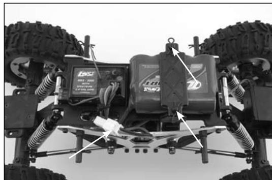
Reinstall the battery strap and body clips. Plug the battery pack into the ESC (fig. 3).
