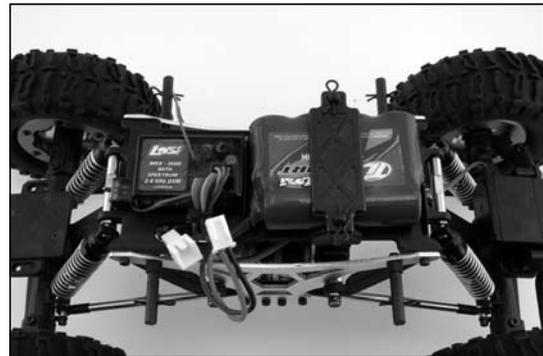
Install the charged battery pack into the chassis as shown (fig.2). Ensure that the battery is laying flat on the chassis.
