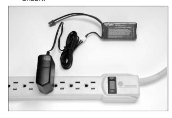
4) Plug the battery into the R.O.S.S. unit in the battery box. Arrange the wires as shown in the photos and replace the battery in the battery box and secure the top with the two wire clips. Plug in the large white plug halves and place the wires into the clips on the top of the cover.
