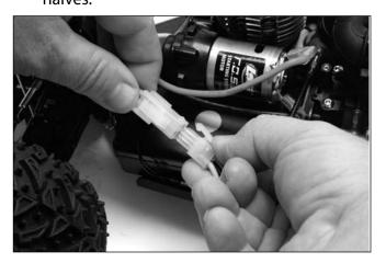
3) Remove the two wire clips holding the top on the battery box and remove the battery pack. Plug the included AC charger into an outlet. Plug the battery pack into the charger noting that it can only be plugged in one way. The light on the charger will glow RED until the battery is charged at which time it will glow GREEN.
