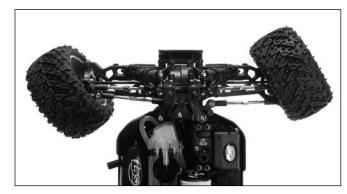
10) Place the model on the ground. Use your thumb to depress the starter button on the back of the transmitter. This will energize the R.O.S.S. starting system. You should be able to see fuel travel from the fuel tank to the carburetor in a few seconds followed by the engine starting to fire.
