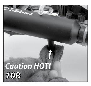
When you are done running your Mega Baja, push the primer button down to stop the engine (fig.10A). It may be necessary to push the primer button down several times. If the engine does not stop, use the handle of a screwdriver or a rag to cover the exhaust pipe exit (fig.10B), being EXTREMELY careful not to burn your hand as this will be hot.
