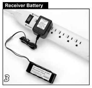
Plug the AC charger into the proper 110V wall receptacle. Plug the charger into the battery pack. When the battery is charging the Red indicator light will be on. A discharged battery will need to be charged for 10-12 hours to attain a full charge.
