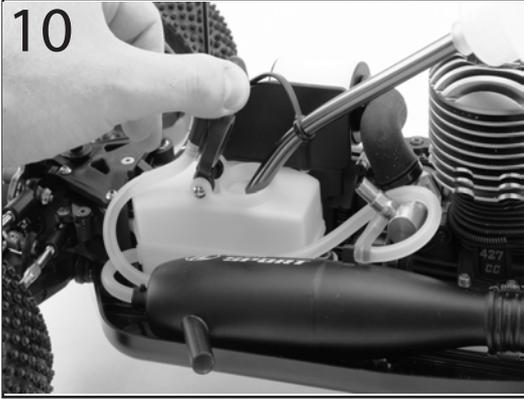
Fill your fuel bottle with fuel and lift the lid of the fuel tank and fill the tank (fig. 10). Make sure to put the lid back on both the fuel bottle and fuel jug.
