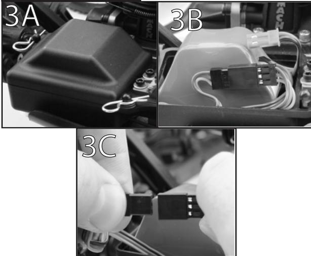
**Note:** Your 8IGHT RTR is equipped with a rechargeable receiver pack installed in your buggy. Follow the instructions to remove or replace the receiver pack.
