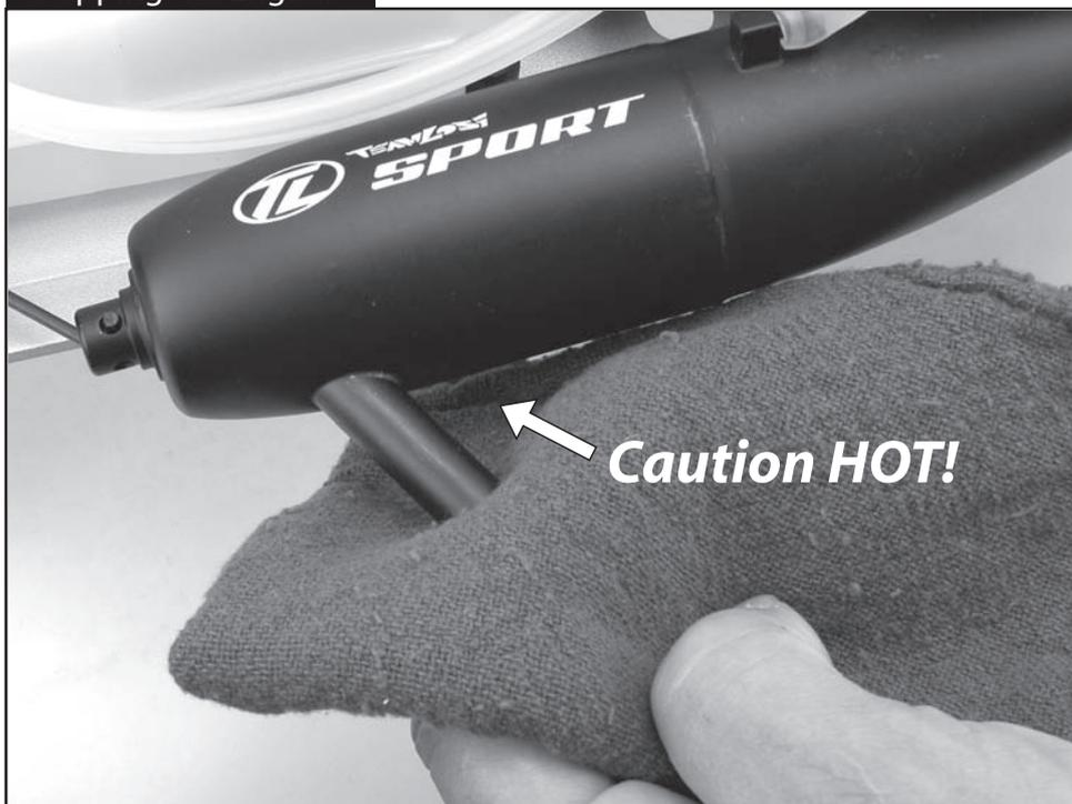
When you are done running your 8IGHT RTR, use the handle of a screw driver or a rag to cover the exhaust pipe exit. Be EXTREMELY careful not to burn your hand as this will be hot. Also, make sure turn the receiver switch off, then turn the transmitter switch off.
