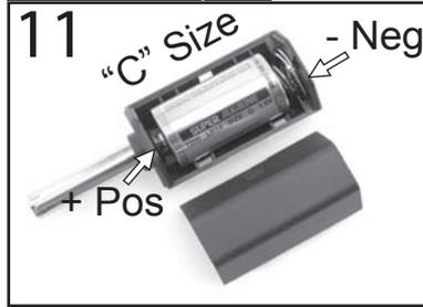
Remove the cover from the Glow plug igniter. Install a "C" size Alkaline battery with the "+" end of the battery as shown.
