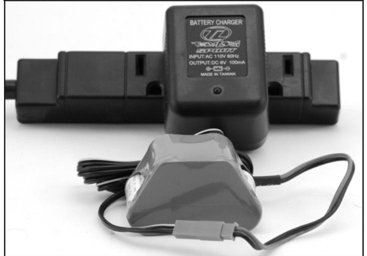
Plug the AC charger into the proper wall receptacle (110V). Plug the red male connector from the battery pack into the red female connector from the charger. When the battery is charging the red indicator light will be on. Charge for 8 to 12 hours depending on the level of charge remaining. Never charge for more than 12 hours. **Never charge the battery with the black battery connector connected to the black switch connector. Damage to your radio system may result.**
