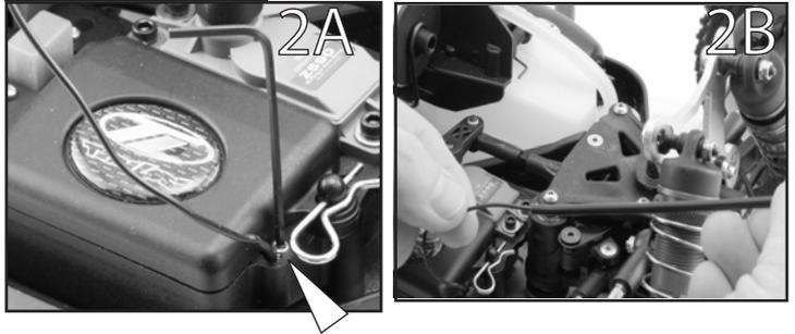
Locate the antenna tube in the plastic bag with the Operations guide. Remove the silver 5-40 setscrew from the radio tray with a 1/16" allen key (fig.2A). Thread the black antenna wire through the antenna tube (fig 2B). Push the antenna tube into the antenna mounting hole, then reinstall the 5-40 setscrew and attach the antenna cap.
