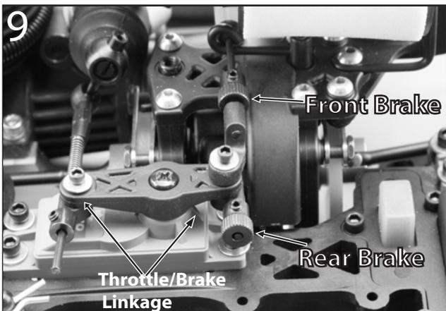
Your 8IGHT RTR is equipped with front and rear adjustable brakes (fig. 9). The upper blue knob adjusts the front brakes and the lower blue knob adjusts the rear brakes. To adjust the brakes turn the blue knob counter-clockwise for more brakes, clockwise for less brakes. These adjustments are for fine tuning and setting the brake bias. You will perform most of your brake adjustments from the transmitter. The collar with the set screw is used to adjust your throttle linkage.
