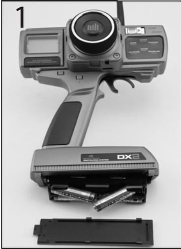
Install the 8 AA-size alkaline batteries in the transmitter making sure the positive(+) and negative (-) ends are oriented correctly. Use only quality alkaline or rechargeable Ni-Cad batteries.
