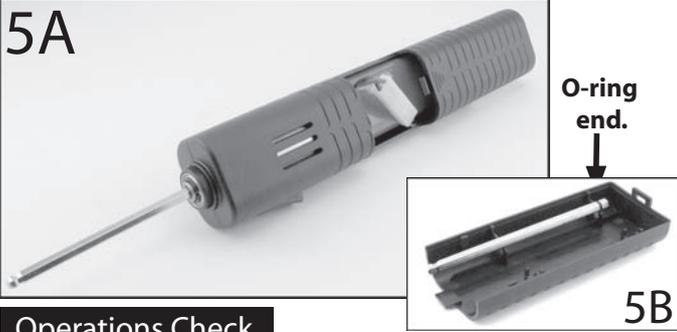
Slide the battery access panel opposite the hand strap back and remove the cover (fig. 5A). Remove hex starter shaft from the back side of the cover, (fig. 5B), and press the o-ringed end into the drive cup. Slide the 6 cell, 7.2 volt, "stick pack" (not supplied), into the Spin-Start and plug it in. Note that the plug is made such that it can only be plugged in one way. Carefully tuck the plug wires under the battery access panel and slide shut.
