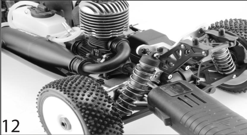
Insert the Spin-Start into the back plate of the engine. Cover the exhaust outlet with a rag. Press the Spin-Start button to turn the engine over for a few seconds. When you see the fuel reach the carburetor, release the Spin-Start button. Excessive priming will flood the engine and make it difficult to start.
