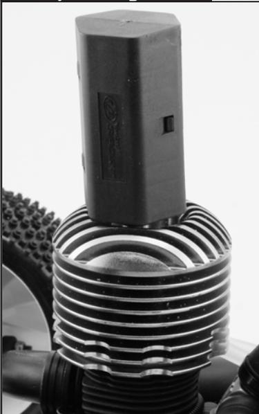
Attach the glow plug igniter to the glow plug. If you are using an aftermarket glow igniter with a meter make sure the needle is in the green or good condition. Holding the starter securely, press on the switch button and the engine should turn over and start.
