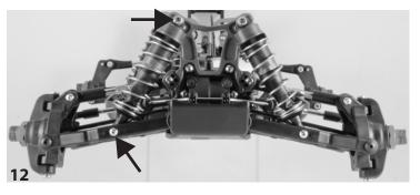
while off-power. **More front and rear droop:** will accelerate better in bumps when going straight, but can cause the truck to traction roll in rough turns. **Less front and rear droop:** will make the chassis slide over bumps better in turns but limit acceleration in the bumps.
