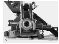
**Less anti-squat:** will produce less off-power steering and allow the chassis to roll (side to side) more across the rear. Less anti-squat will help the chassis accelerate better in small bumps.
