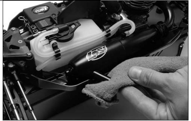
To stop the engine, use the handle of a screwdriver or a rag to cover the exhaust pipe exit (fig.), being **EXTREMELY** careful not to burn your hand as this will be hot.
